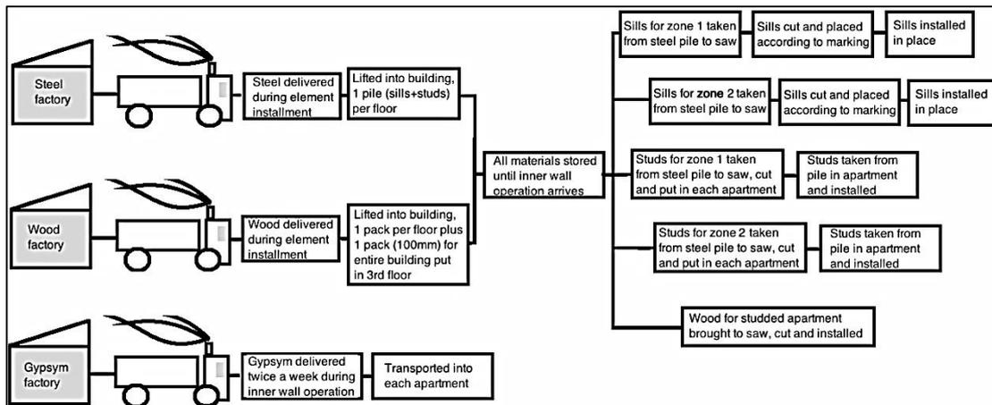
Figure 3: Process Map for all materials, initial operation
