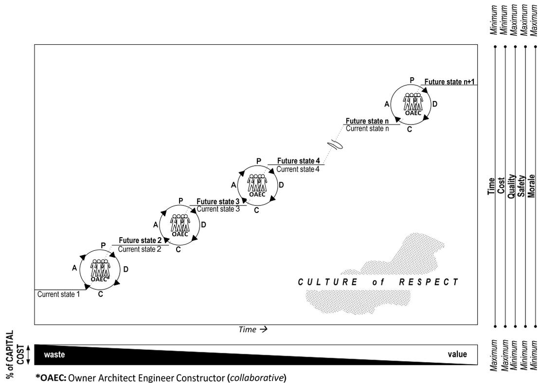
Figure 1: The continuous improvement process of lean construction (after Rybkowski et al. 2013, Figures 4 & 5, p. 88).
