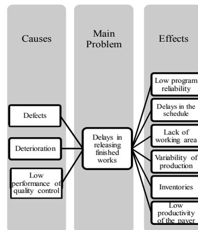
Figure 5: Root-Cause diagram
