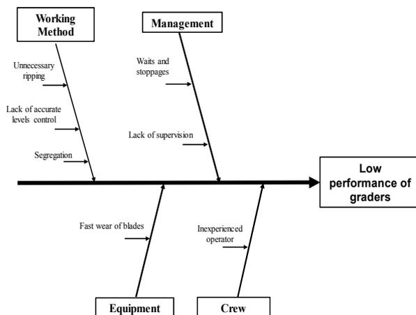
Figure 4: Cause-and-effect diagram
