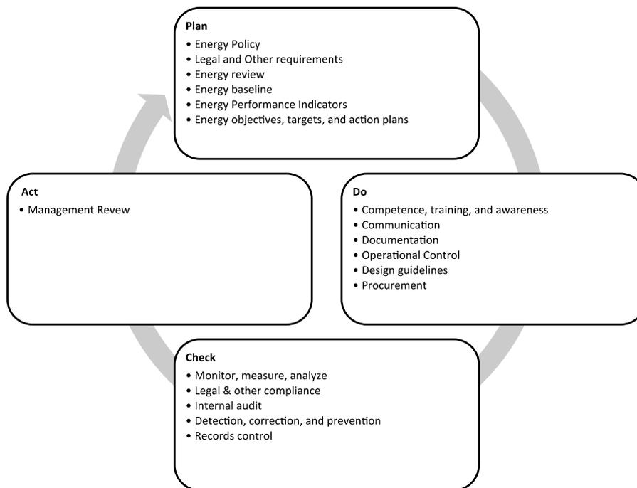
Figure 1. Energy Management System Requirements mapped to the Plan-Do-Check-Act Cycle
