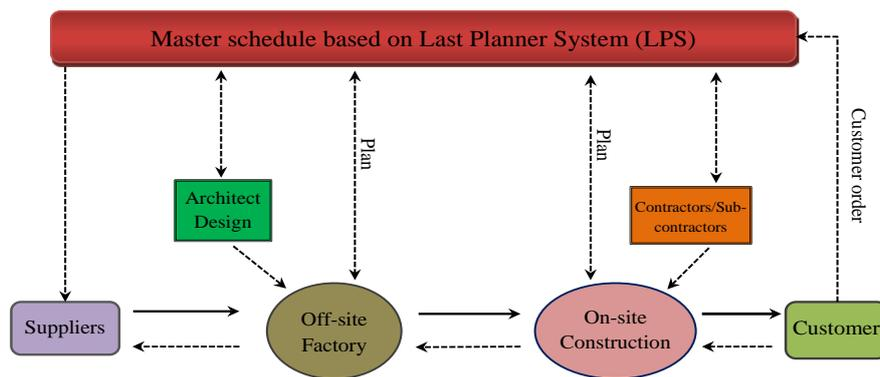
Figure 1: Conceptual model of prefabricated house building SC.
