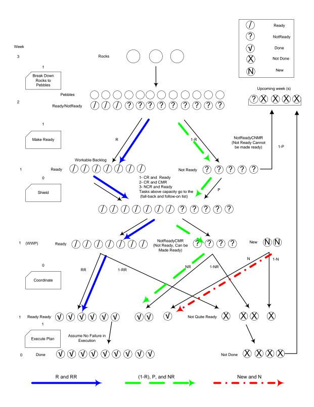
Figure 3: Possible paths that tasks take from the lookahead plan to the weekly work plan (Hamzeh 2009)
