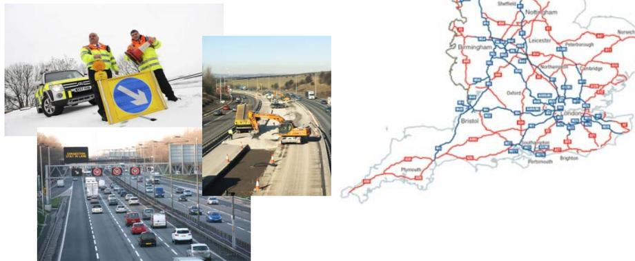
Figure 1 – The Motorways (in blue) and Trunk Roads (in red) which forms the HA Strategic Road Network
