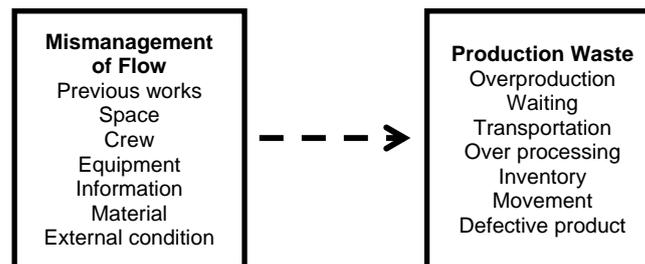
Figure 2: Relationship between Mismanaged Flows and Production Waste Adapted from (Koskela 2000) and (Ohno 1988)
