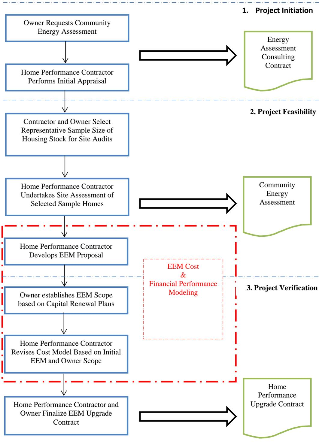
Figure 2: Typical Energy Improvement Retrofit Process
