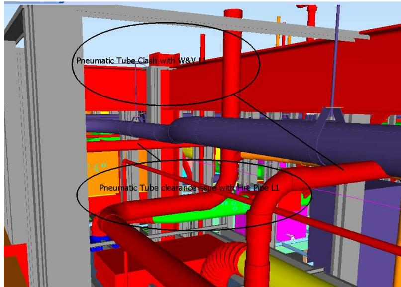
Figure 2: Hard Clash between Pneumatic Tube (purple) and Waste and Vent (W&V, red), and Soft Clash between Pneumatic Tube (purple) and Fire Pipe (red)
