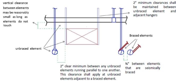
Figure 4: Component clearances (Source: Eric Osterling, Unger Construction)
