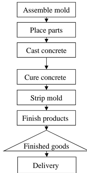
Figure 1: Precast production process
