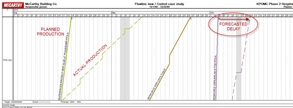
Figure 3: The forecasted delay of reinforcing due to staging conflicts between pier cap rebar and waterproofing
