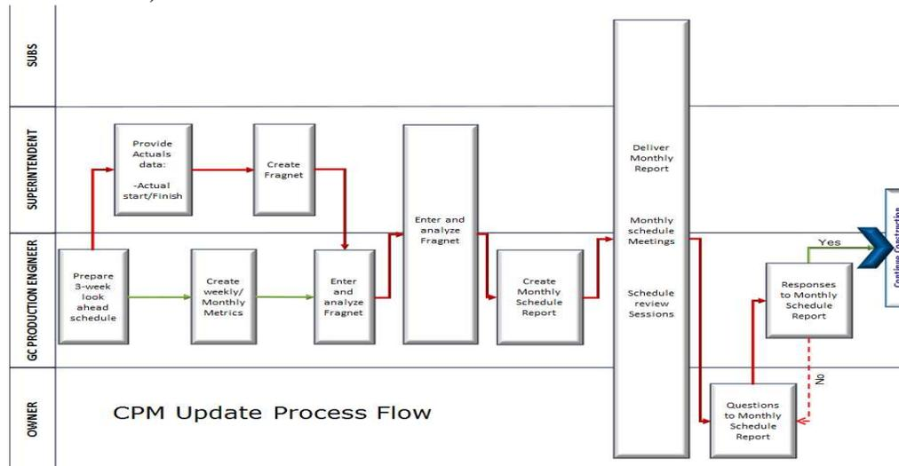
Figure 1: The process flow for the CPM updating process used on the hospital project
