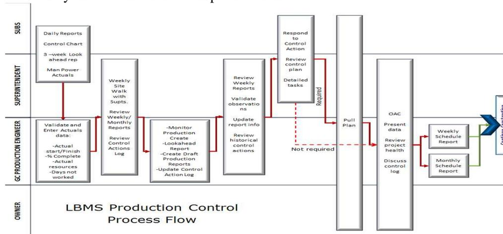
Figure 2: The LBMS process flow for production control on the hospital project
