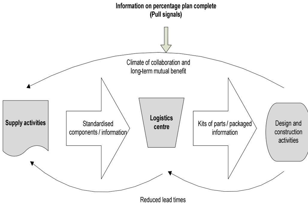
Figure 1: Lean supply system suitable for construction logistics management (source: Terry and Smith 2011: 147).
