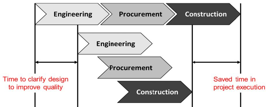
Figure 1: Sequential versus Concurrent EPC (Emblemsvåg 2012)
