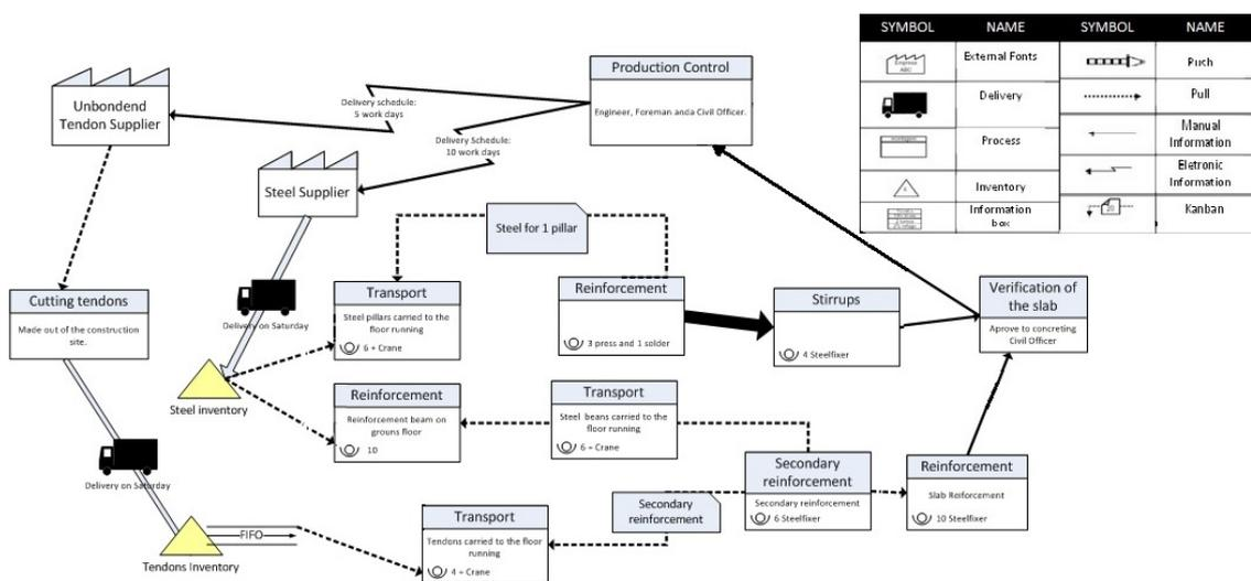
Figure 12: Value Stream Mapping of Future state for the macro case.
