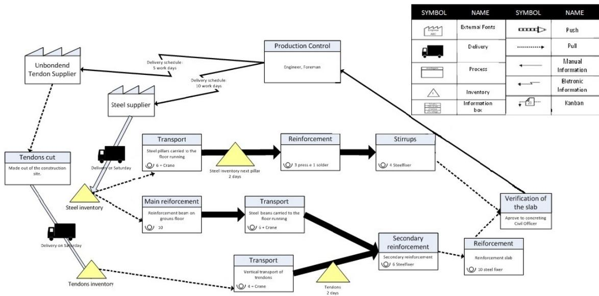
Figure 10: Current Value Stream Mapping of the macro case.
