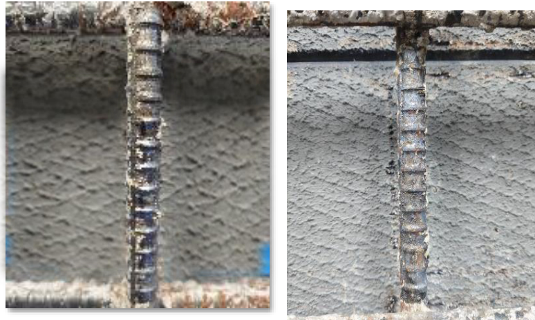
200W Laser 100W Laser Figure 13: Compare of 200W Laser and 100W Laser
