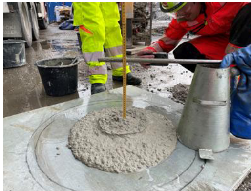
Figure 1: Controlling the workability of the fresh concrete
