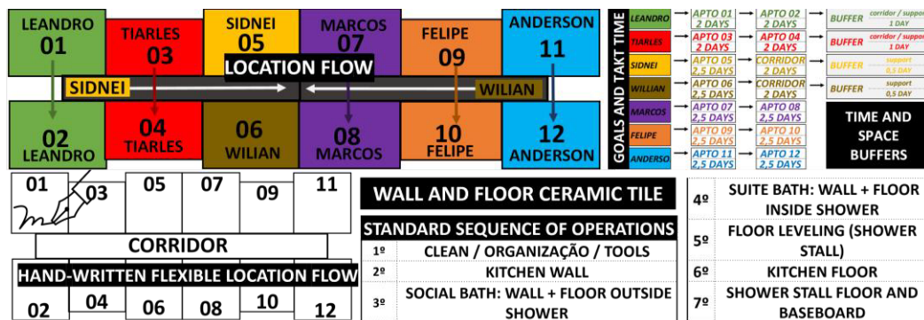
Figure 6: (1) Visual device that displays batch sizes, workers allocation and location flow, apartment takt time, time and space buffers and standard activity sequence; (2) Example of flexible allocation visual device.
