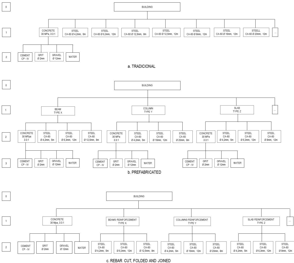
Figure 3: BOMs reflecting different construction methods
