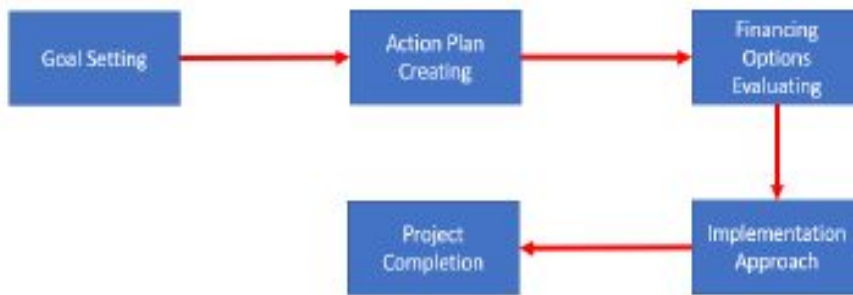
Figure 1: Energy retrofit process recommended by U.S. Department of Energy, created based on the energy retrofit guide (Hendron, R.; Leach, M.; Bonnema, E.; Shekhar, D.; Pless, 2013)
