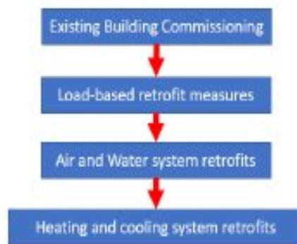
Figure 2: A staged approach to Energy Efficiency Upgrades recommended U.S. Department of Energy, created based on the energy retrofit guide (Hendron, R.; Leach, M.; Bonnema, E.; Shekhar, D.; Pless, 2013)
