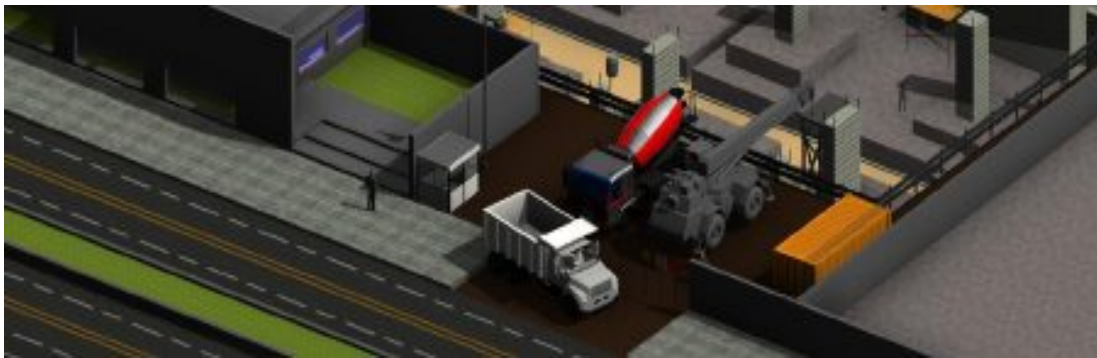
Figure 13: Primary material un-loading and concrete pumping point
