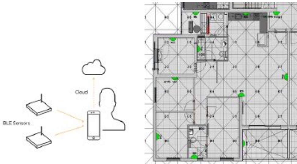
Figure 3 BLE tracking system components Figure 4 Typical beacon placement in a residential building
