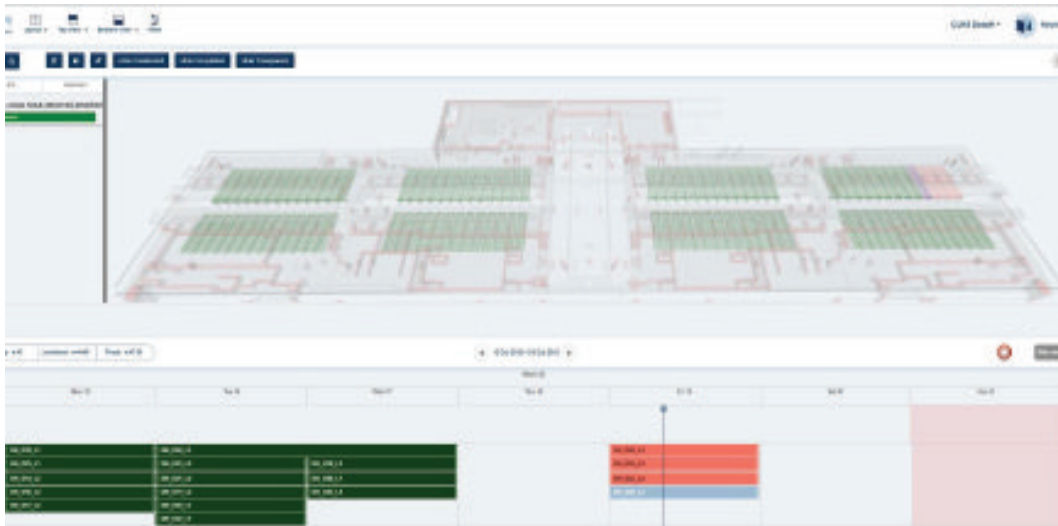
Figure 27 Integrated production plan with BIM in VisiLean.
