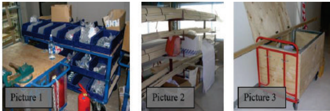
Figure 53 Examples from a project that challenged with the principle "everything on wheels". Picture 1 Both workstation and part storage, picture 2 Larger trolleys used for electrical tubes, metal stud and mouldings. Picture 3. More standard solution. (Photo: J.S)
