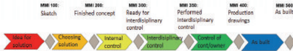
Figure 62: Flow sheet made by Fløisbonn et al. (2018) that should work as a base for a design process using MMI in a Norwegian building project
