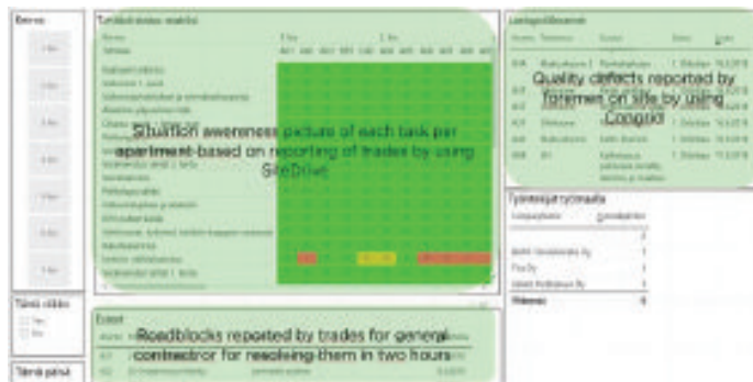
Figure 2. Situation awareness tool (Fira Insite), which was developed during the project for site manager and foremen for visualising the current status of tasks and roadblocks as reported by trades.
