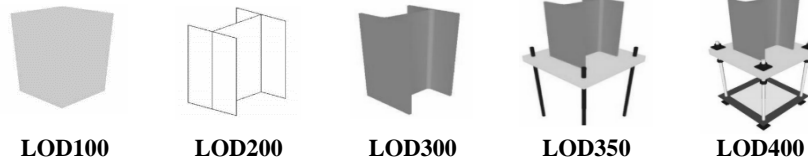
Figure 1: Visual illustration of LOD-levels for a column (BIMForum 2017)
