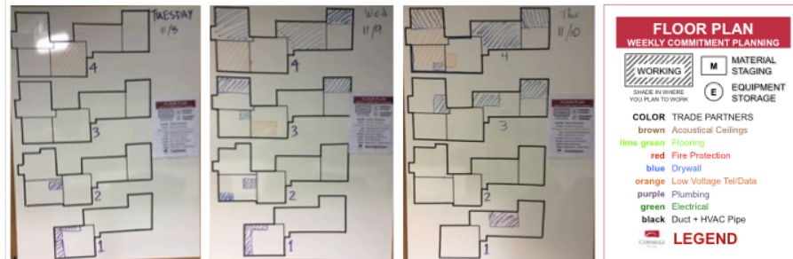
Figure 3: Floor Plan Boards used for Weekly Commitment Planning and Materials Management on an Office Renovation Project
