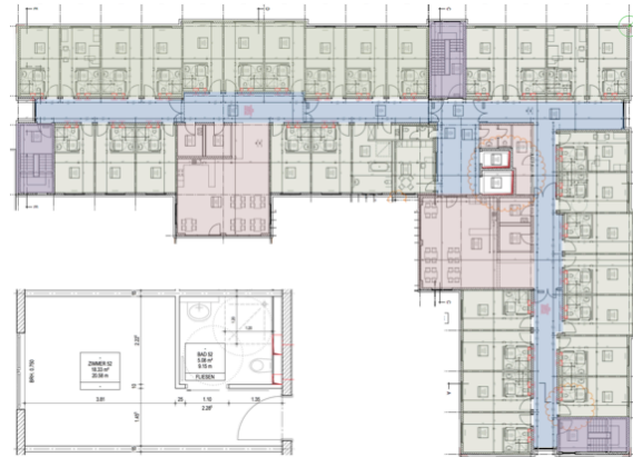
Figure 1: Floor plan using colours to show functional clusters to define the interior fit-out and the SSU of a habitable room.
